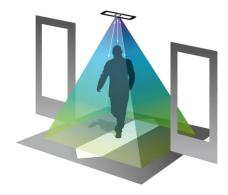
The field of view is determined by the aperture angles of the time-of-flight sensor.
