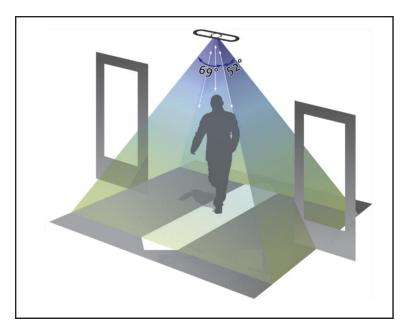
The field of view is determined by the aperture angles of the time-offlight sensor. With aperture angles of 69° (in the direction of the door width) and 52° (in the direction of passenger movement), the covered door width results from the mounting height of the sensor, as shown in the table.
