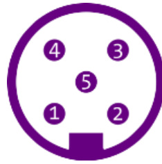
M12 Power (male, a-coded, 5 pin)
