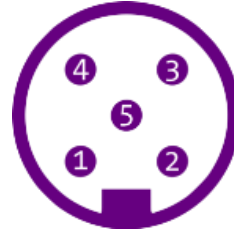
M12 Power (male, a-coded, 5 pin)
