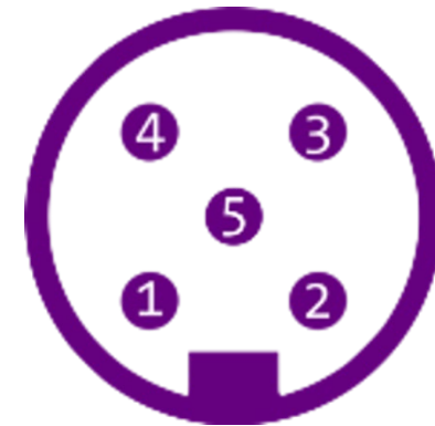
M12 power supply, typ. 24 V (male, a-coded, 5 pin)
